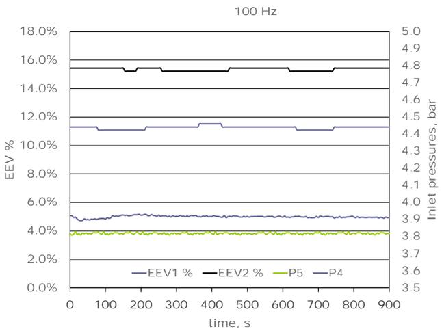
Fig. 12: Experimental results on electronic expansion valves working in parallel: 100 Hz.
