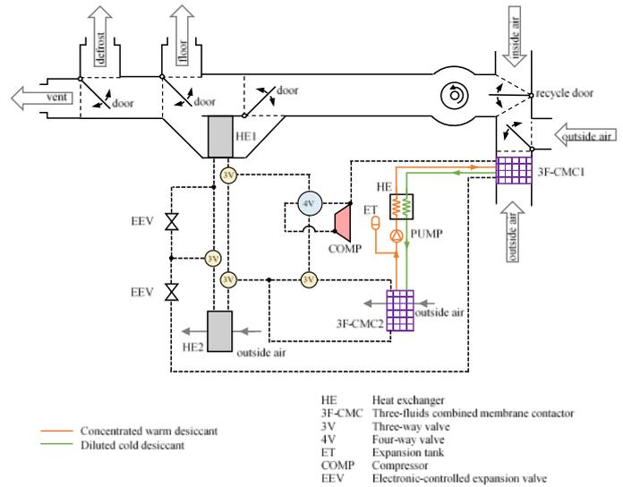
Fig. 2: XERIC climate-control system architecture.
