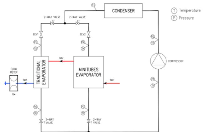
Fig. 10: Scheme of the refrigeration testing cycle.
