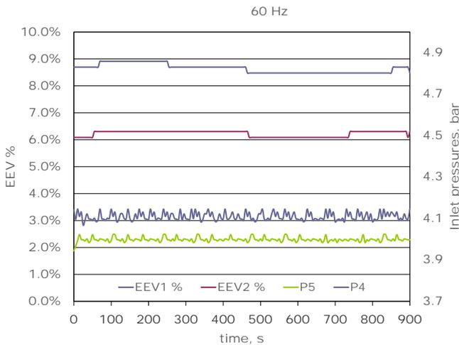
Fig. 11: Experimental results on electronic expansion valves working in parallel: 60 Hz.
