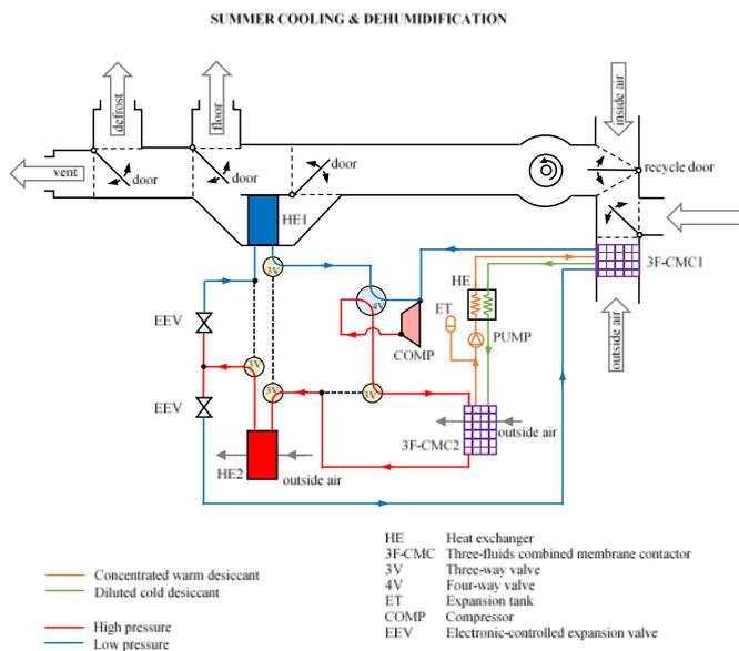
Fig. 3: Summer cooling & dehumidification action.
