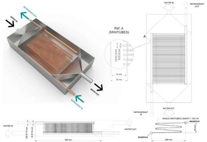
Fig. 9: Schematic view of the mini tubes heat exchanger.
