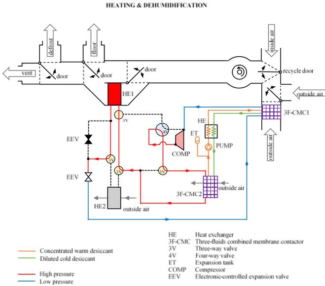
Fig. 6: Air dehumidification & heating.
