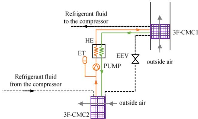
Fig. 1: Sketch of the desiccant loop that uses two 3F-CMCs.
