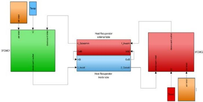
Fig. 8: Simulink scheme representing the desiccant loop.
