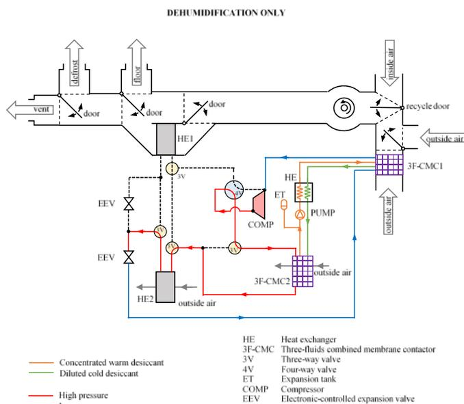
Fig. 5: Air dehumidification.
